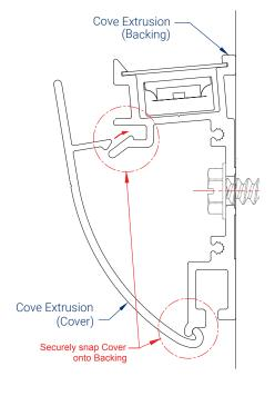
NOTE: Cover must snap onto Backing
