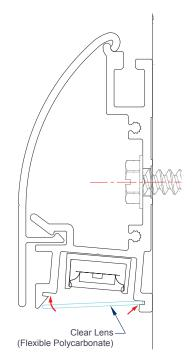
**NOTE**: Test LED strip prior to installing lens. Press fit flexible lens as shown.
