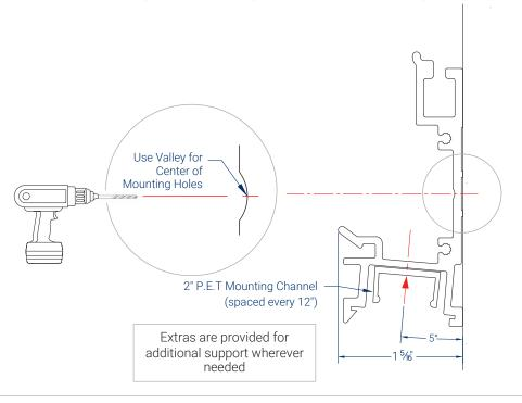
2 ORGALED LED INSTALLATION · GENTLY PUSH-FIT THE ORGALED LED STRIP INTO THE P.E.T. MOUNTING CHANNEL. Mounting holes per contractor Appropriate mounting hardware to be provided per Contractor 2" P.E.T Mounting Channel OrgaLED LED Strip
