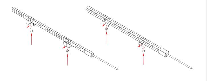
NOTE: BE CAUTIOUS OF LED STRIP BENDING. THIS WILL DAMAGE THE STRIP.
