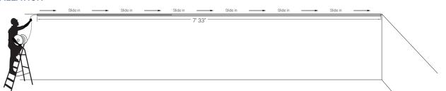
1 Use double-sided adhesive under the Mounting Tab or 6-32 screws (by others) to mount OrgaGlide 1® Channel to surface.
