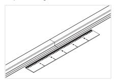
3 Install OrgaGlide 1<sup>®</sup> Channels with a 2" gap for Bi-directional feeds.
