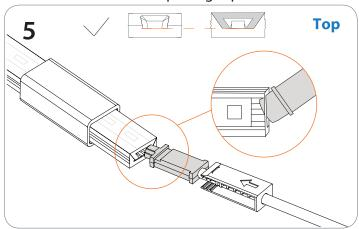
Slide the Top connector (3) sideways into the hollow chamber of the OrgaLED® LED strip.
