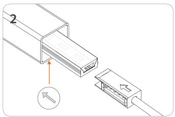
Take into account the direction of the arrow on the bottom of the OrgaLED® LED strip and align it with the arrow on the clamp (4).
