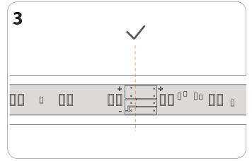
**Top view** | Make sure the cut is vertical as illustraded in the image above. Only cut on the dotted lines to prevent damaging the LED strip.
