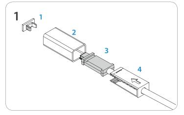
The OrgaLED® IP40 Connector consists of: End cap (1), Shell (2), Connector (3), Clamp (4).
