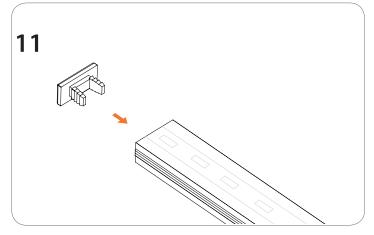
Finish the connection by inserting an end cap (1) in the hollow chamber on the end side of the OrgaLED® LED strip.
