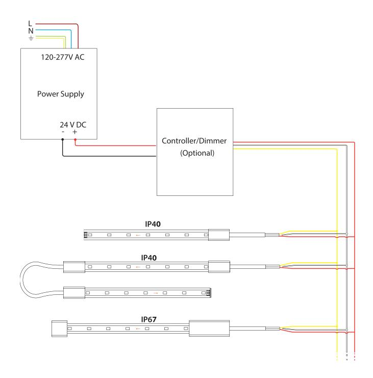
Connect the LED strip as indicated in the figure above. The wires should be connected as follows: Red (+) and Black (-).
