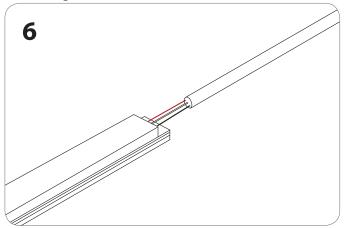
Connect the OrgaLED® LED strip to the power supply (24 V DC) constant voltage.
