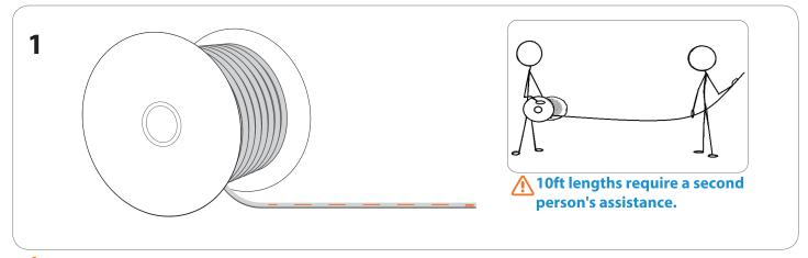
The LED strip has to be unreeled on a horizontal surface at the time of installation. Do not unreel the spool of LED strip before installation. Lengths over 10ft should be installed with the help of a second person to support the strip to ensure that the connector is not stressed.
