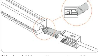
**Side view** | Make sure the connector and the PCB are perfectly horizontally alligned.
