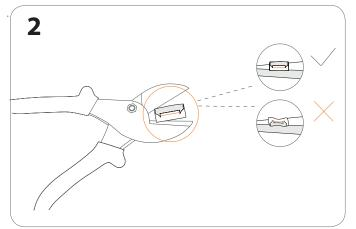
Place the OrgaLED® LED strip on the base of the cutting tool. Not doing so may result in a deformed LED strip.
