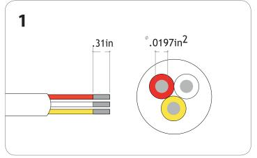
Solder the wires to the PCB. We advise to use a cable with an area not higher then 0.02 in.
