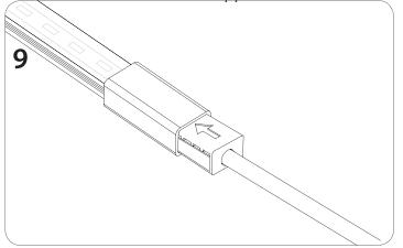
Test the OrgaLED® LED strip before you slide it fully over the clamp (4).
