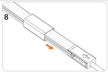
Slide the shell (2) partly over the clamp (4).
