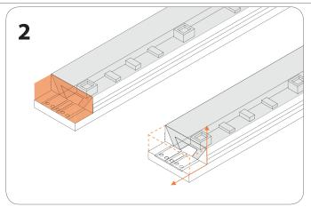
**Top view** | Only cut the LED strip extrusion on the dotted line of the extrusion to prevent damaging the PCB. Carefully cut this part of the extrusion, we recommend folding up to use as a cover once the solder is finished.
