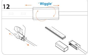
\*\*Uninstalling the connector multiple times may weaken the connection point over time. To remove 'wiggle' the connection from the LED and pull apart in the opposite direction. Do **not** pull on the cord.
