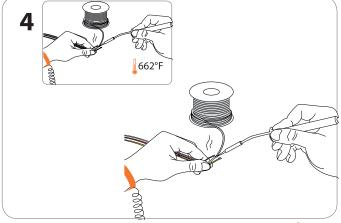
Pre-solder the connector pads before soldering the wires.
