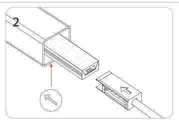
Take into account the direction of the arrow on the bottom of the OrgaLED<sup>®</sup> LED strip and align it with the arrow on the clamp (4).
