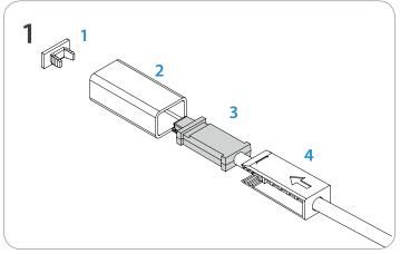
The OrgaLED<sup>®</sup> IP40 Connector consists of: End cap (1), Shell (2), Connector (3), Clamp (4).
