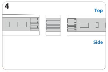
**Top view** | Make sure the cut is vertical as illustraded in the image above. Only cut on the dotted lines to prevent damaging the LED strip.
