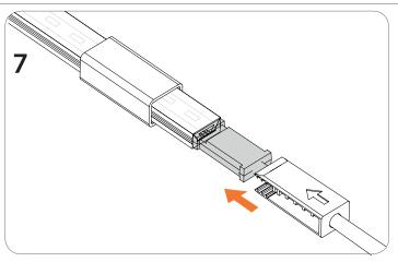
Slide the clamp (4) over the connector (3) and make sure that the arrow is on the upper side.
