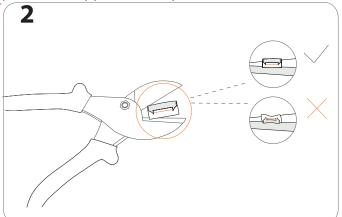
Place the OrgaLED<sup>®</sup> LED strip on the base of the cutting tool. Not doing so may result in a deformed LED strip.
