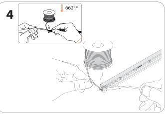
Pre-solder the connector pads before soldering the wires.
