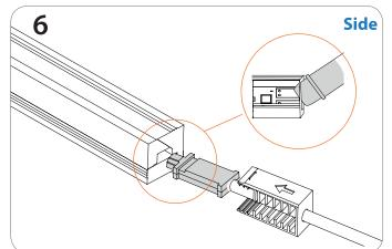
**Side view** | Make sure the connector and the PCB are perfectly horizontally alligned.
