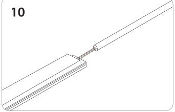
Connect the OrgaLED<sup>®</sup> LED strip to the power supply (24 V DC) con-stant voltage.
