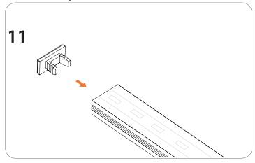
Finish the connection by inserting an end cap (1) in the hollow chamber on the end side of the OrgaLED<sup>®</sup> LED strip.
