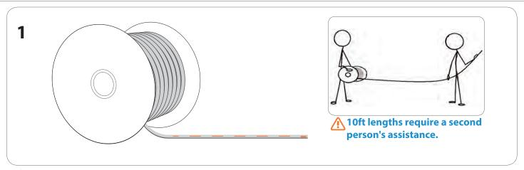
The LED strip has to be unreeled on a horizontal surface at the time of installation. Do not unreel the spool of LED strip before installation. Lengths over 10ft should be installed with the help of a second person to support the strip to ensure that the connector is not stressed.
