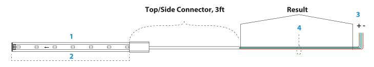
**Result** = Maximum cable length based on the cable thickness and power supply voltage.
