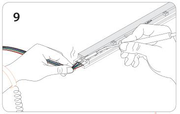
Solder the wires to the connector pads, making sure the solder does not flow out of the pad areas, which could cause a short.
