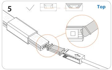
Slide the Top connector (3) sideways into the hollow chamber of the liniLED<sup>®</sup> LED strip. Side view | Do not cut the PCB!
