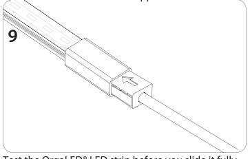
Test the OrgaLED<sup>®</sup> LED strip before you slide it fully over the clamp (4).
