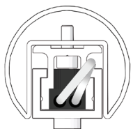
cross section with power cables
