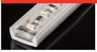
Specification grade waterproof flexible linear LED light strip providing the illumination levels of high output LEDs from multiple miniature LEDs for very low energy (< 3W/ft.). No UV or IR. liniLED® can be applied both indoors and outdoors. Co-extruded with built in reflectors the highly flexible UV stabilized, optically clear PVC seals the LEDs for permanent protection against adverse environments and handling. Rapid mounting in long runs with "Solder free" push-fit connections.
